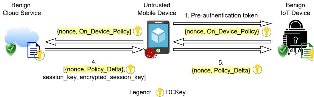
Figure 5: Secure Access Policy Synchronization (SAPS) Protocol
