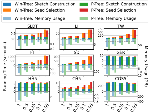
Figure 7: Running time and memory with different values of \alpha . The x-axis represents the compression rate. The growing up y-axis represents the running time (in seconds) of the sketching and selecting process. The growing down y-axis represents the total memory usage (in GB). The gray horizontal line represents the CSR size of each graph, which is the basic memory we need to load the graph.
