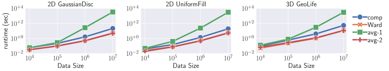
Figure 8: Runtimes (seconds) of our algorithm “PC” on three data sets of varying sizes using 48 cores with two-way hyper-threading. The “Ward” and “avg-2” lines overlapped because they have similar runtimes. The results show that the scalability is very similar across datasets.
