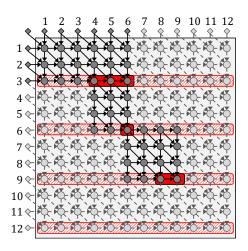
**Figure 1** Example square grid and path sketch for M' = 3 and h = k = 4. The circles are nodes in the square. The diamonds are input nodes (outputs of adjacent squares), omitting irrelevant edges. The red slashes are the 4 superrows, and the solid red are the sketch segments.
