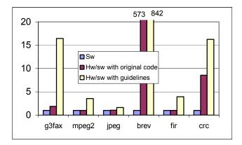
Figure 4: Speedups of hardware/software solution compared to software both without and with coding guidelines.
