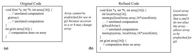
Figure 2: *Pass-by-value return* for arrays. a) The array used in function g() cannot be prefetched during f() because the pointers a and b may modify elements of the array. b) Copying the array into a local array guarantees that a and b are not aliases, allowing the array to be prefetched into on-chip memory before execution of g().
