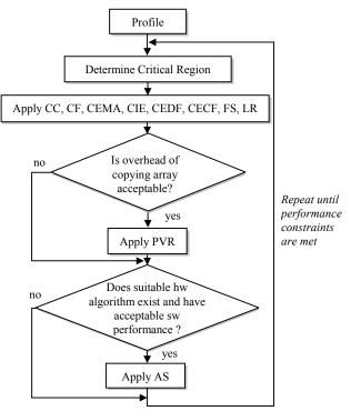
Figure 3: Methodology for applying coding guidelines to achieve hardware performance improvements while minimizing software overhead.
