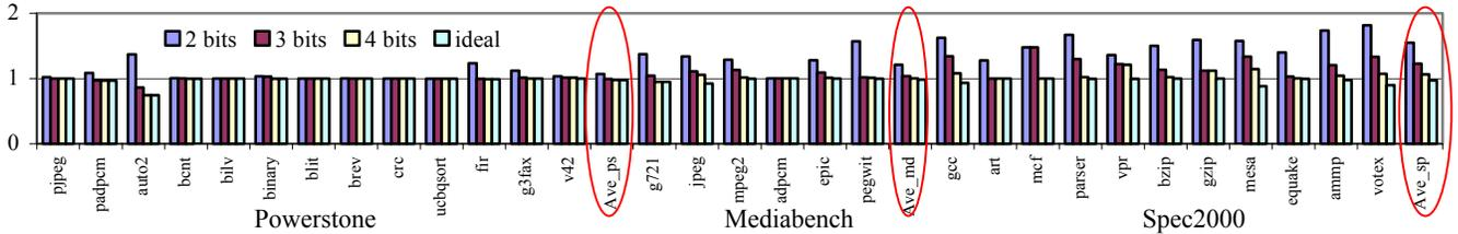
Figure 2: Average number of ways of instruction cache activated when 2-bit, 3-bit, and 4-bit are compared in parallel with address decoder. *Ave\_ps*, *Ave\_md*, and *Ave\_sp* stand for average of Powerstone, Mediabench, and Spec 2000 respectively.
