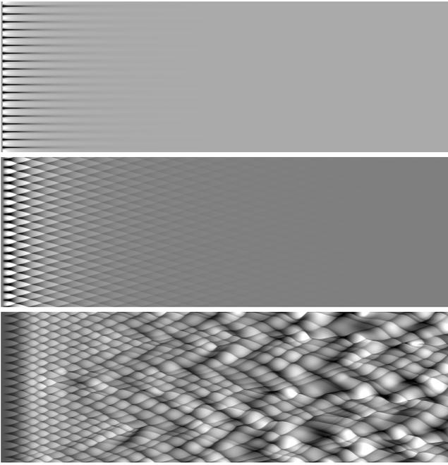
Figure 2: Simulated smoked foils. Lighter regions correspond to a slower flame speed, and the flame moves from left to right in each figure. An initial sine wave perturbation is smoothed out by the first order DSD equations (top) and the second order DSD equations (middle), whereas interesting cellular patterns develop for the third order DSD equations (bottom).
