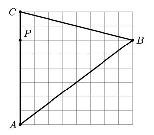
16. Give a detailed algorithm for determining if a ray intersects an axis-aligned box in 2D. Assume the box has left, right, bottom, and top edges at  $x = x_{\min}$ ,  $x = x_{\max}$ ,  $y = y_{\min}$ ,  $y = y_{\max}$ , respectively. Let the ray be given by  $\mathbf{r}(t) = \mathbf{e} + t\mathbf{u}$ ,  $t \ge 0$ . An example case is depicted below.
