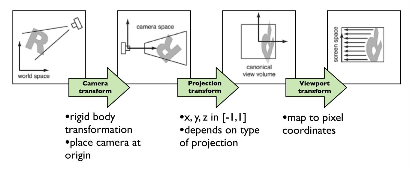
Viewing transforms depend on: camera position and orientation, type of projection, field of view, image resolution
