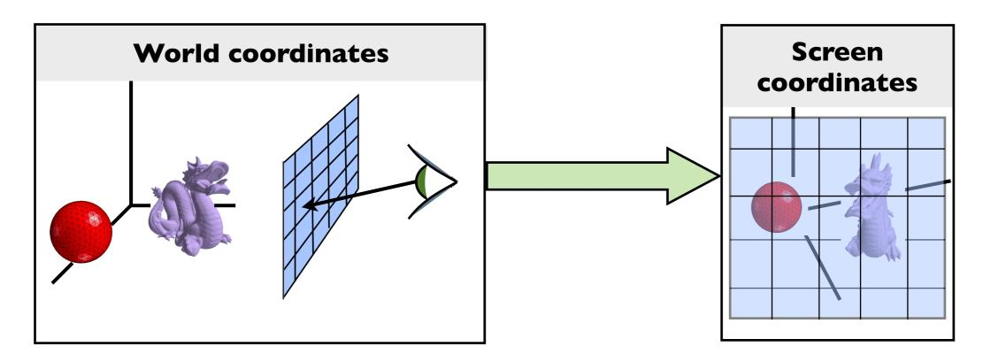
The viewing transformation also projects any point along the pixel's view ray back to the pixel's position in **image space**
