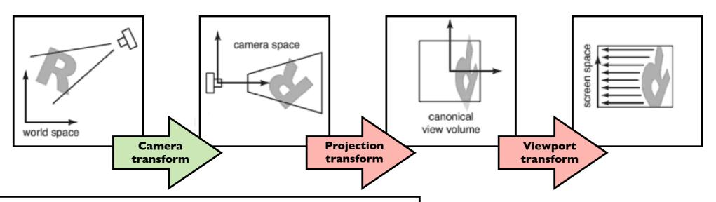
$$\begin{aligned} & \text{construct } M_{vp} \\ & \text{construct } M_{orth} \\ & M = M_{vp} M_{orth} \\ & \text{for each line segment } (a_i, b_i) \, \text{do} \\ & \mathbf{p} = M \mathbf{a}_i \\ & \mathbf{q} = M \mathbf{b}_i \\ & \text{drawline } (x_p, y_p, x_q, y_q) \end{aligned}$$
