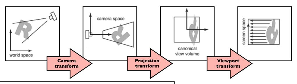
$\begin{aligned} & \text{construct } M_{vp} \ M_{cam} \\ & \text{construct } M_{orth} \\ & M = M_{vp} M_{orth} M_{cam} \\ & \text{for each line segment } (a_i, b_i) \, \text{do} \\ & \mathbf{p} = M \mathbf{a}_i \\ & \mathbf{q} = M \mathbf{b}_i \\ & \text{drawline } (x_p, y_p, x_q, y_q) \end{aligned}$
