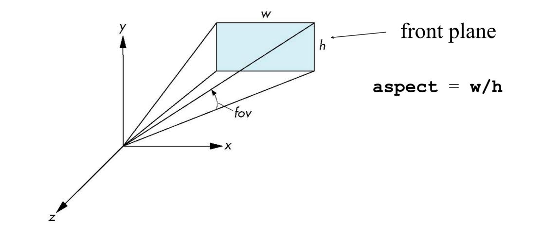
Sometimes it's more convenient to just give an angle, the field-of-view, and an aspect ratio, instead of I, r, t, b. The glu library provides such a function. It will figure out I, r, t, b, and call glFrustrum for you.
