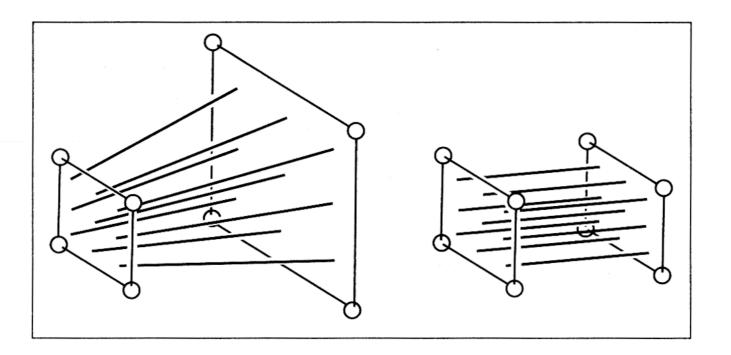
So far we've mapped the view frustrum to a rectangular box. This rectangular box has the same near face as the view frustrum. The far face has been mapped down to the far face of the box. This mapping is given by P. The bottom figure shows how lines in the view frustrum get mapped to the rect. box.
