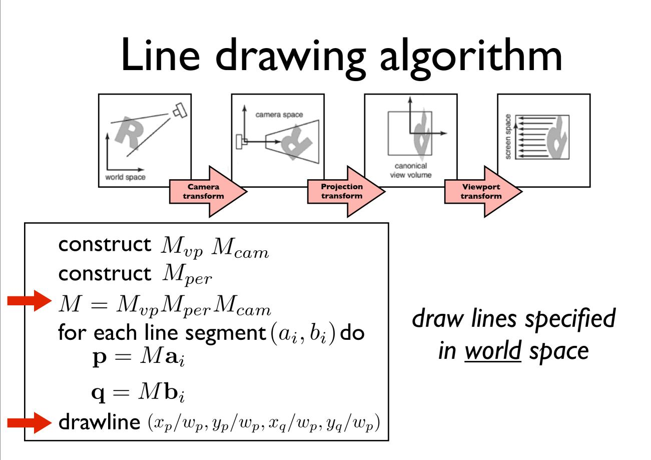
Note the two lines that have changed: 1. we put our perspective transformation into the overall transformation matrix M. 2. When we call the drawline function, we have to divide the x and y coordinates by the w coordinate.
