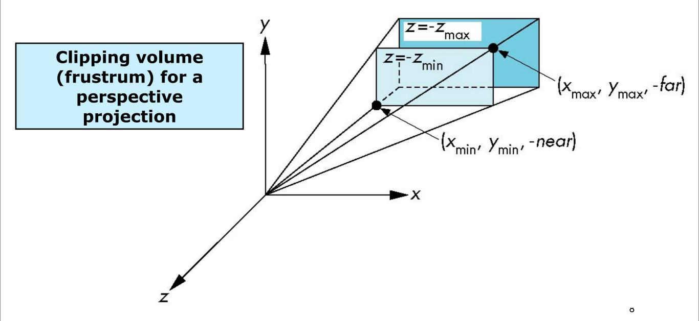
Here's how you set up a perspective view in OpenGL. Note that near and far are both negative, but you pass their absolute values to OpenGL. Another difference with OpenGL is that it uses a left-handed coordinates system after the camera transformations.
