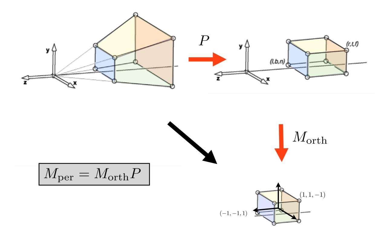
We need a second mapping to get our points into the canonical view volume. This second mapping is a mapping from one box to another. So it's given by an orthographic mapping, M\_orth. The final perspective transformation is the composition of P and M\_orth.
