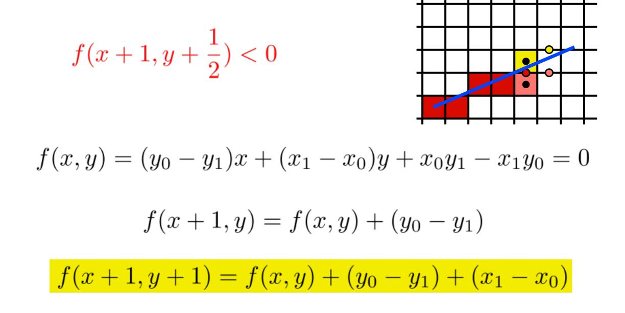
′ = y0 d = f(x0+1,y0+1/2)for x = x0 to xI do draw(x,y)if (d<0) then y = y + |d = d+(y0-y1)+(x1-x0)else d = d + (y0 - y1)
