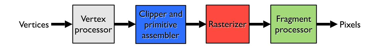
clipping - clip objects to viewing volume rasterization - make fragments from clipped objects hidden surface removal - determine visible fragments
