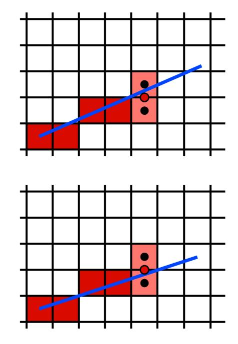
y = y0for x = x0 to x1 do draw(x,y) if  $(f(x+1, y+\frac{1}{2}) < 0)$  then y = y+1
