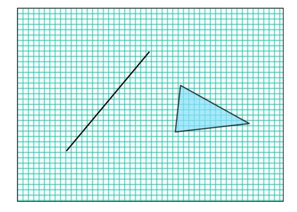
Rasterization is the process of determining which pixels are "covered" by the primitive
