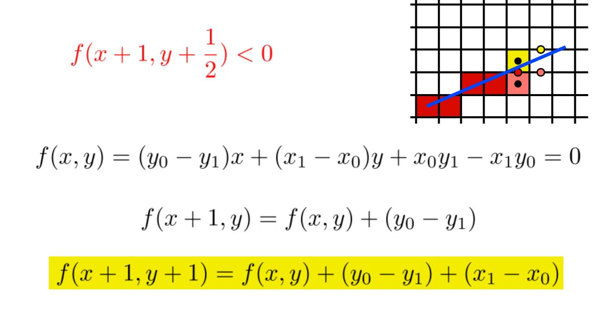
y = y0 d = f(x0+1,y0+1/2)for x = x0 to xI do draw(x,y)if (d<0) then y = y + |d = d + (y0 - y1) + (x1 - x0)else d = d + (y0 - y1)
