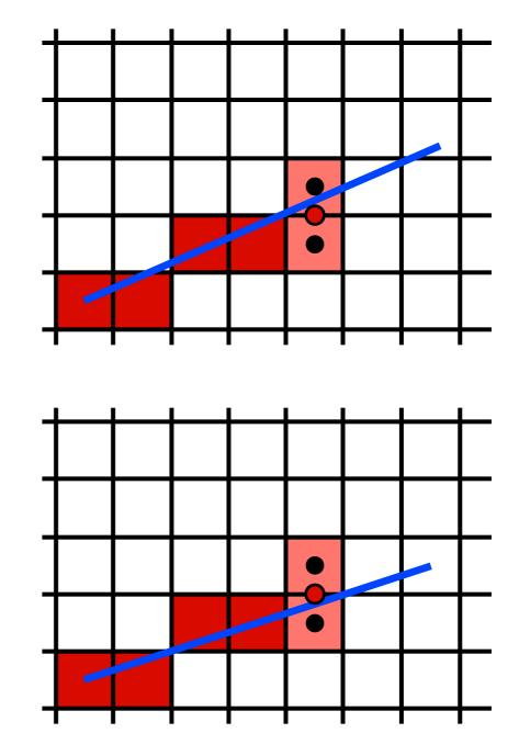
y = y0for x = x0 to x1 do draw(x,y) if ( $f(x+1, y+\frac{1}{2}) < 0$ ) then y = y+1
