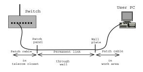
Figure 2: Detailed view of a single link segment.
