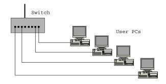
Figure 1: Four hosts having dedicated access to four ports of a switch
