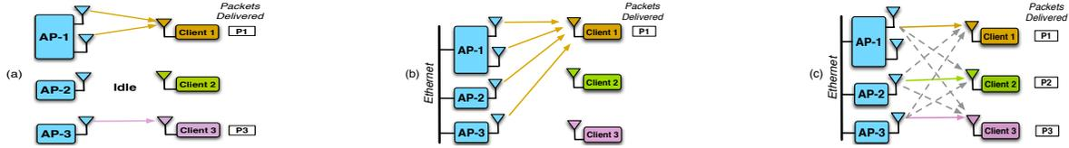
Figure 1 (a) Reuse: Two slot schedule: AP1, AP3 active simultaneously in slot 1, AP2 in slot 2. (b) DAS: 3 slot schedule - 3 APs sending same data to one client in each slot. (c) netMIMO: 3 APs sending 3 data streams to 3 clients in each slot.
