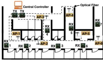
Figure 8 : Testbed deployment
