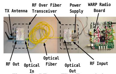
Figure 7 : RF over Fiber Transmission
