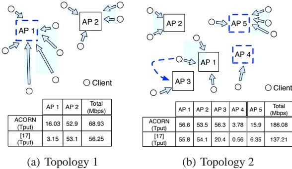
**Figure 10: ACORN can provide throughput gains in interference-free deployments. Dashed APs use 20 MHz with ACORN and 40 MHz otherwise. Dashed arrows depict the user affiliation decisions taken by [17].**
