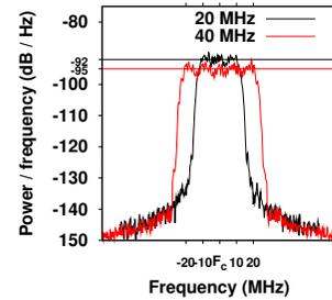
Figure 1: PSD estimate with different channel widths.
