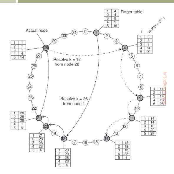
Resolving key 26 from node 1 and key 12 from node 28 using DHTs in Chord (using finger tables)
