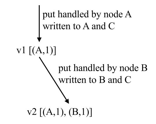
$v_2 > v_1$ , so Dynamo automatically drops  $v_1$  at C
