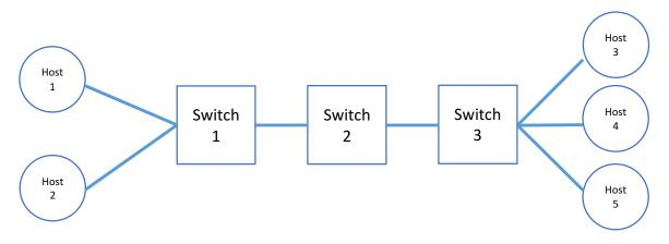
In Parts A and B, all traffic will be directed to the network controller, which will make decisions on behalf of the switches. In Parts C and D, the controller will install rules on the switches so they can forward traffic themselves.
