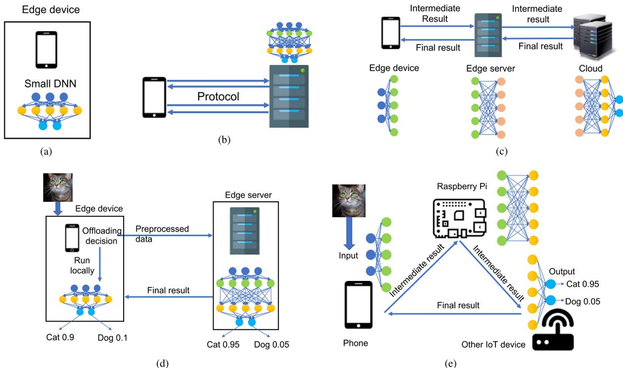
**Fig. 5. Architectures for deep learning inference with edge computing. (a) On-device computation. (b) Secure two-party communication. (c) Computing across edge devices with DNN model partitioning. (d) Offloading with model selection. (e) Distributed computing with DNN model partitioning.**
