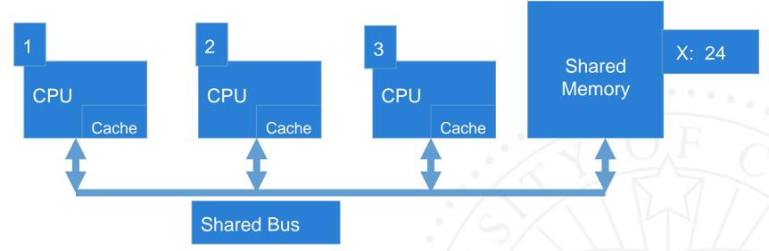
Processor 1 reads X: obtains 24 from memory and caches it Processor 2 reads X: obtains 24 from memory and caches it Processor 1 writes 32 to X: its locally cached copy is updated Processor 3 reads X: what value should it get? Memory and processor 2 think it is 24 Processor 1 thinks it is 32
