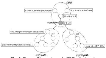
Fig. 5: The condition-path graph (CPG) of a branch.
