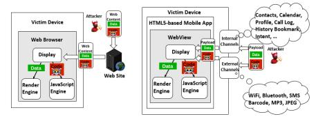
(a) XSS attack on Web Applications (b) Code Injection Attack on HTML5-based Apps Figure 2: Code Injection Attacks on Web Applications and HTML5-based Mobile Apps
