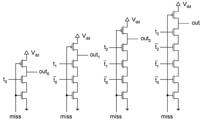
Fig. 22. Single priority selector circuits.
