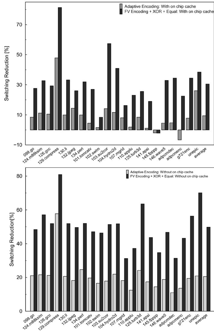
Fig. 29. FV versus adaptive encoding.
