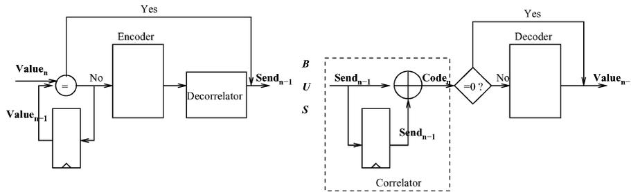
Fig. 6. Dealing with equal code transfer.
