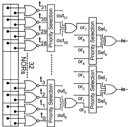
Fig. 23. Timestamp registers and priority selectors circuits.
