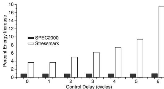
Figure 15: Impact of sensor delay on energy.
