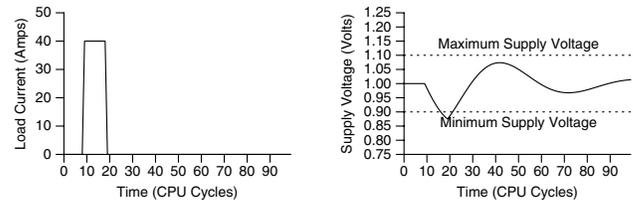
Figure 4: Response to a wide current spike.
