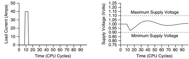
Figure 3: Response to a narrow current spike.
