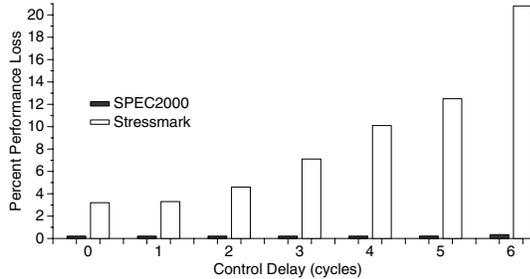
Figure 14: Impact of sensor delay on performance.
