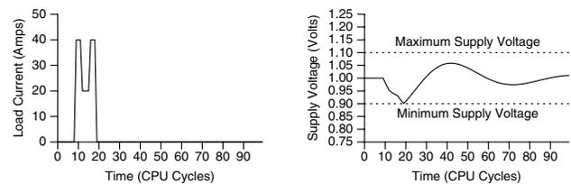
Figure 5: Response to a notched current spike.
