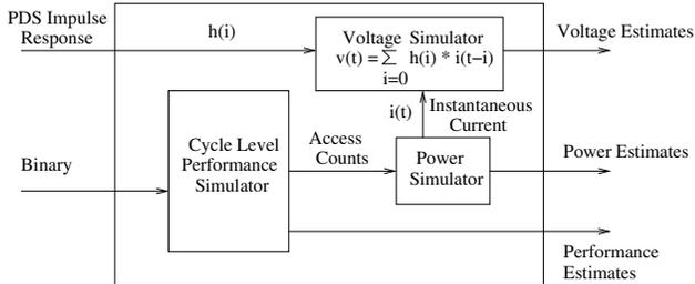
Figure 7: Voltage simulation
