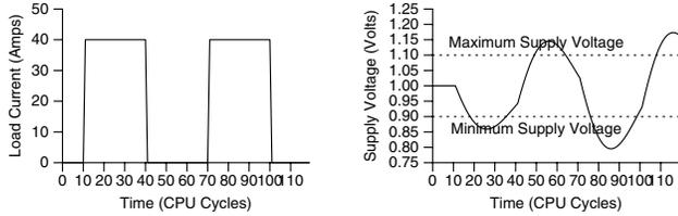
Figure 6: System response to pulses at resonant frequency.
