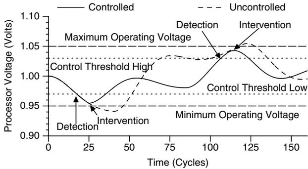
Figure 11: A simple threshold controller in action.
