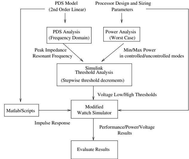
Figure 13: Design flow for microarchitectural voltage control.
