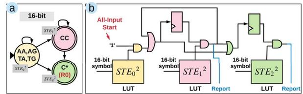
Fig. 3. Automata mapping in LUT-based design.
