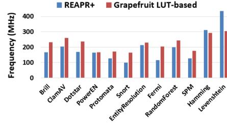
Fig. 7. Comparing Grapefruit (8-bit) with REAPR+ [29].
