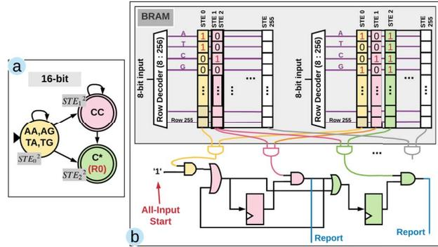
Fig. 4. Automaton mapping in BRAM-based design.
