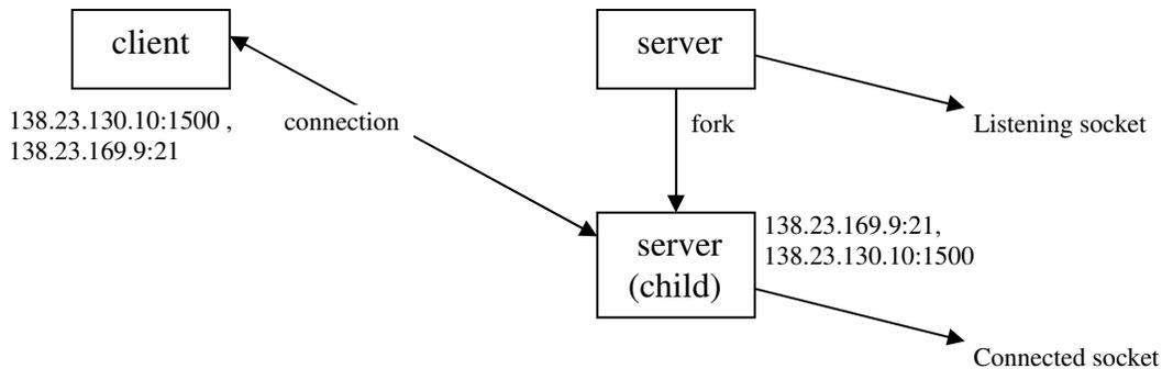
**Figure 2: Server fork()s a copy of itself and lets the child handle this client from port 21, but it concurrently keeps listening (by the parent process) from port 21 as well.**
