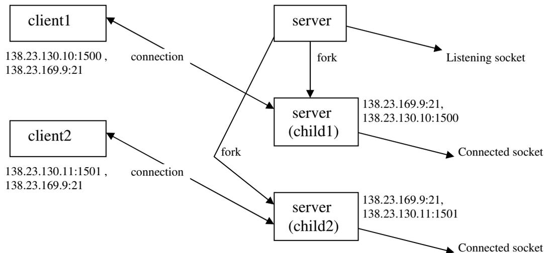
**Figure 3: Another client requests to connect to this server. The server fork(s) another copy of itself and lets this second child handle this client, whereas it still concurrently keeps listening from port 21 (by the parent process) and keeps serving client1 from port1 (by the first child process).**
