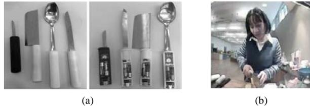
Figure 10. a) Modified Wii Remotes embedded in specially designed utensils. b) A subject is preparing salad. This figure is used with permission from [33].
