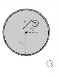
(a) The height of  $m_2$  is  $r_2 \sin \theta$ , so its potential energy is  $r_2 m_2 g \sin \theta$ . The height of  $m_1$  is  $y_0 + r_1 \theta$ , where  $y_0$  is its height when  $\theta = 0$ . The total potential energy is then  $\phi = r_2 m_2 g \sin \theta + (y_0 + r_1 \theta) m_1 g$ . Since a constant shift in potential energy does not matter, we can write
