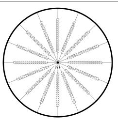
(a) The springs have zero rest length but are free to rotate at both ends. Formulate a force law for one of the springs. That is, express  $\mathbf{f}$  in terms of the mass position  $\mathbf{x}$ , assuming the other end of the spring is fixed at  $\mathbf{z}$ . (If your force does not work with the calculations below, choose a new one.)
