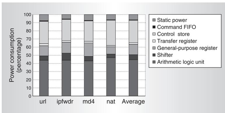
Figure 7. Microengine power consumption breakdown, by component.
