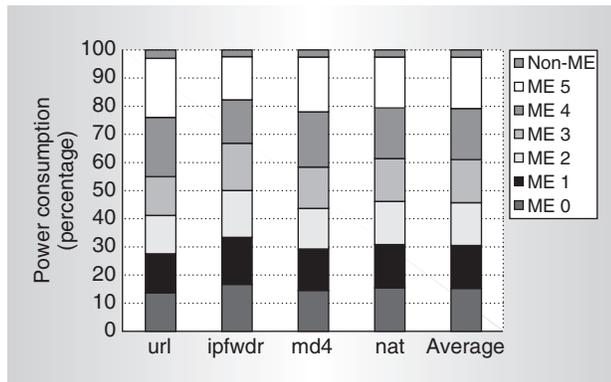
Figure 6. Simulated IXP1200 power consumption breakdown among microengines.
