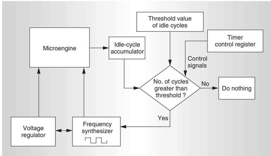
Figure 10. Dynamic voltage scaling (DVS) policy control mechanism.
