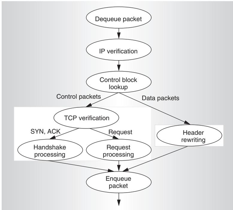
Figure 7. Data flow on the clientME.
