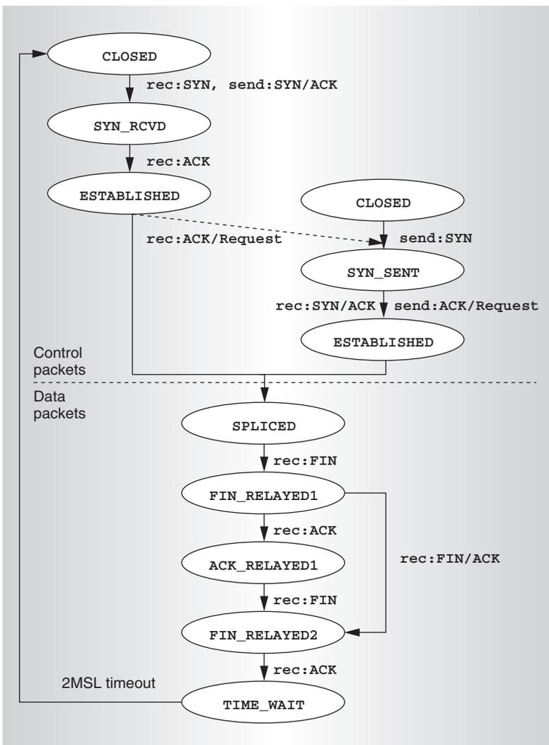
Figure 4. State transition in TCP splicing.
