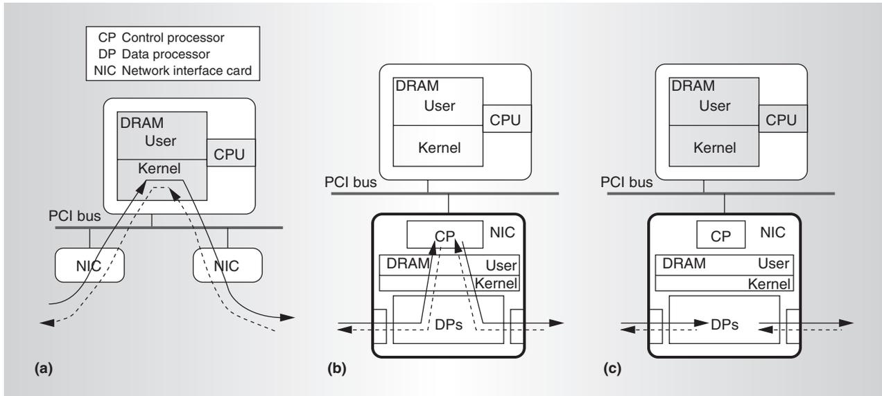
Figure 2. Three architecture candidates for a content-aware switch: Linux-based interface in which processing occurs in the kernel space (a); network-processor-based interfaces in which processing occurs in the control processor (b) as well as in the data processor (c).
