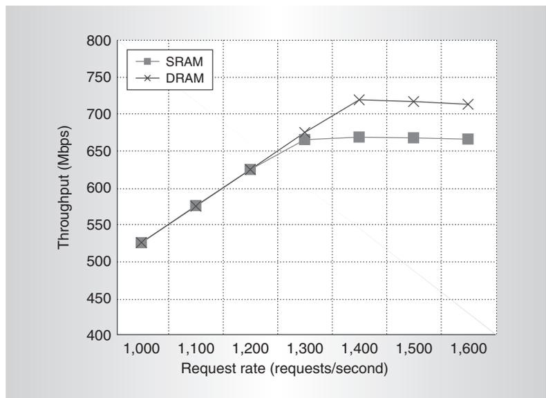
Figure 10. Throughput comparison for control blocks implemented in SRAM and DRAM.
