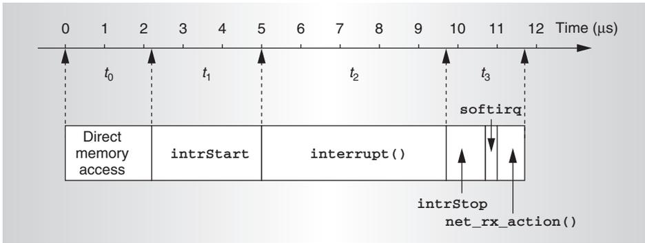
Figure 3. Direct-memory-access and interrupt handling for receiving a 41-byte packet through TCP/IP in a Linux machine.
