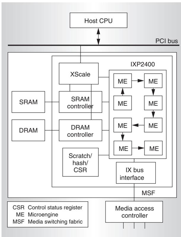
Figure 5. ENP2611 high-level architecture.
