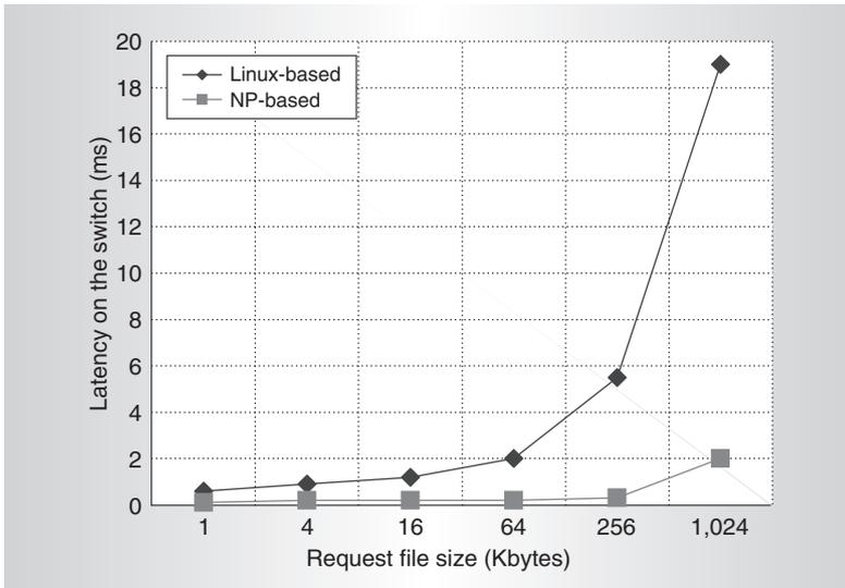
Figure 8. Latency in a Linux-based switch versus an NP-based switch for an HTTP session.
