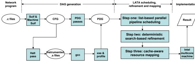
Figure 1: LATA system design flowchart.
