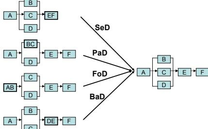
**Figure 6:** Illustration of four decomposition techniques. Thick boxes indicate bottleneck nodes.
