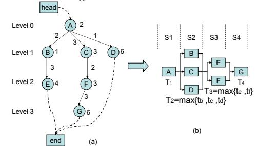
Figure 2: Parallel pipeline scheduling from a DAG.
