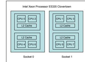
**Figure 8:** Layout of two Quad-Core Intel Xeon E5335 processors.
