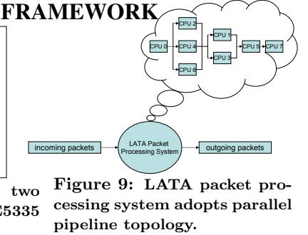
**Figure 9:** LATA packet processing system adopts parallel pipeline topology.
