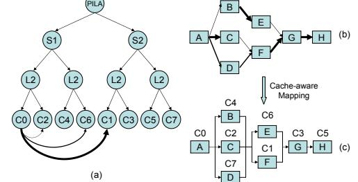
**Figure 7:** The hierarchy of processing units (PUs) on Xeon chip with communication asymmetry and illustration of cache-aware mapping.
