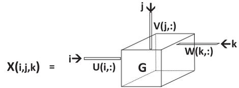
Fig. 5. Element-wise view of the Tucker model.
