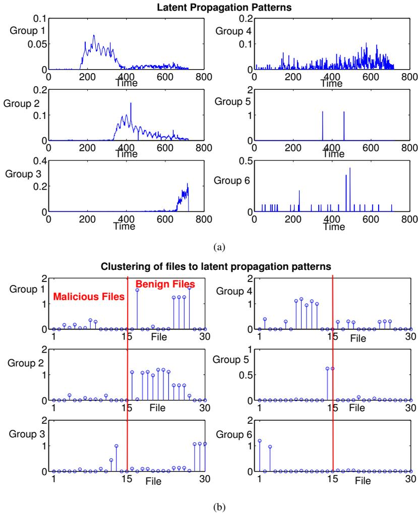
**Fig. 9** Latent representation of the propagation pattern, and clustering of the time series, before sampling. In both subfigures, the vertical axis represents the degree of participation of each data point to the particular Group/Co-cluster. In subfigure (a) the horizontal axis is time and in subfigure (b) the horizontal axis is the file ID.
