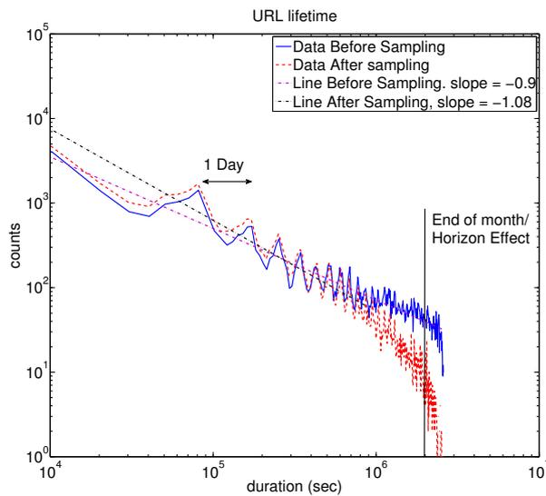
**Fig. 8** Distribution of URL lifetimes, before and after sampling, in log-log scale. The lifetime of URLs follows the PPL model, which is a periodic power law distribution with slope -1 and daily periodicity. We also show the end of June 2011, which signifies the end of our measurement period and thus the start of the horizon effect.
