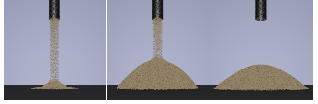
Figure 8: Sand pours into a pile. Our reflection boundary conditions handle the frictional collisions with the ground.
