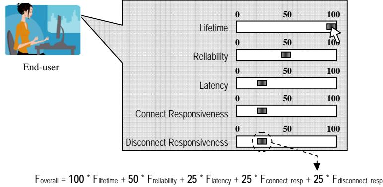
**Figure 5:** End-users utilize a web-based interface to specify the relative importance of each design metric. Individual weights are assigned by setting the corresponding slide switch to the desired position. Each design metric weight is then combined into an overall objective function.
