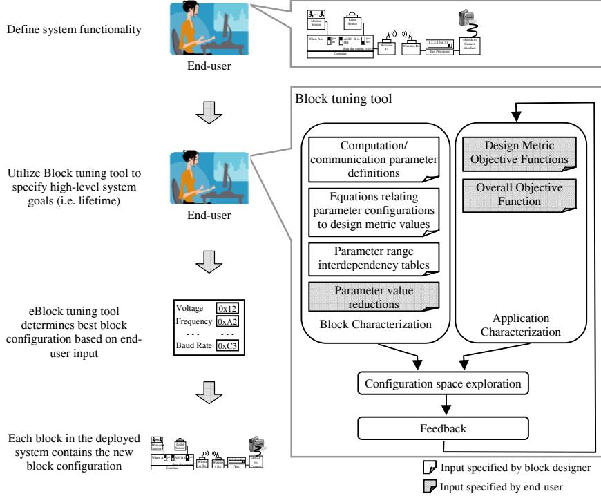
**Figure 2:** Block tuning tool overview. A block designer performs block characterization once.
