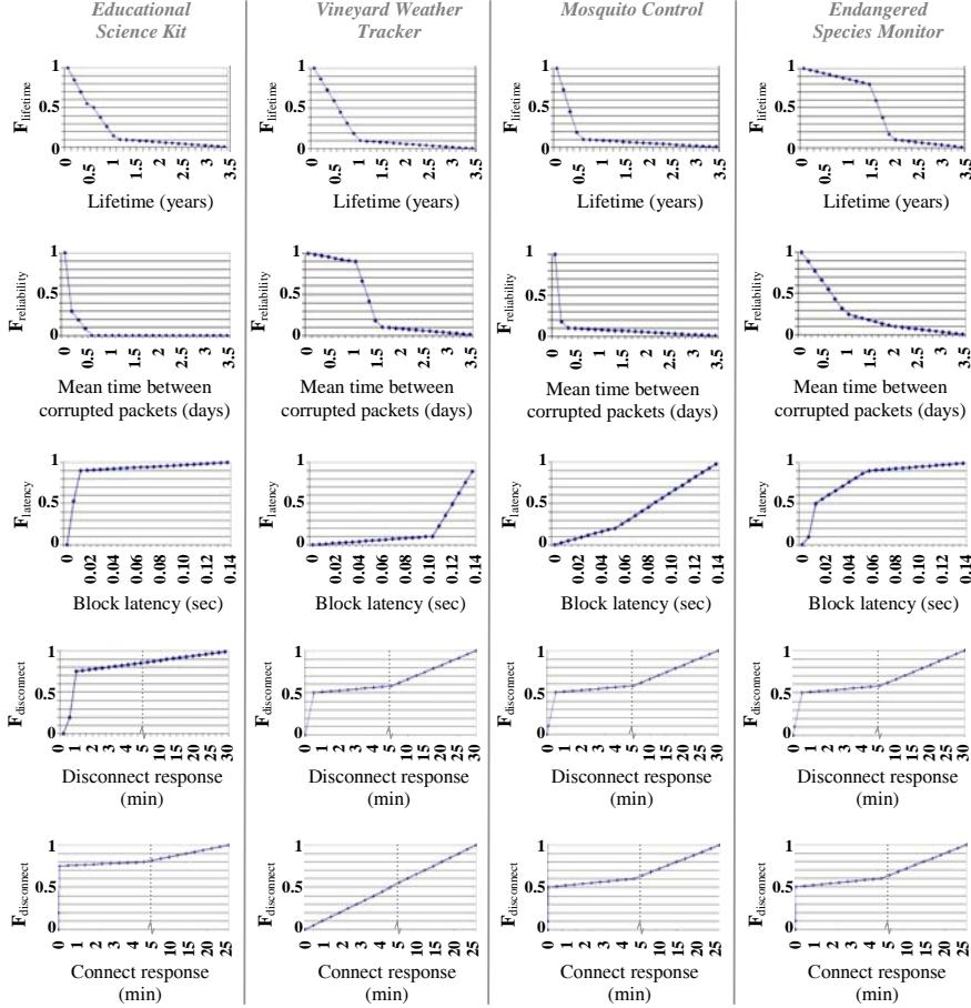
**Figure 6:** End-user defined design metric objective functions for four different applications.
