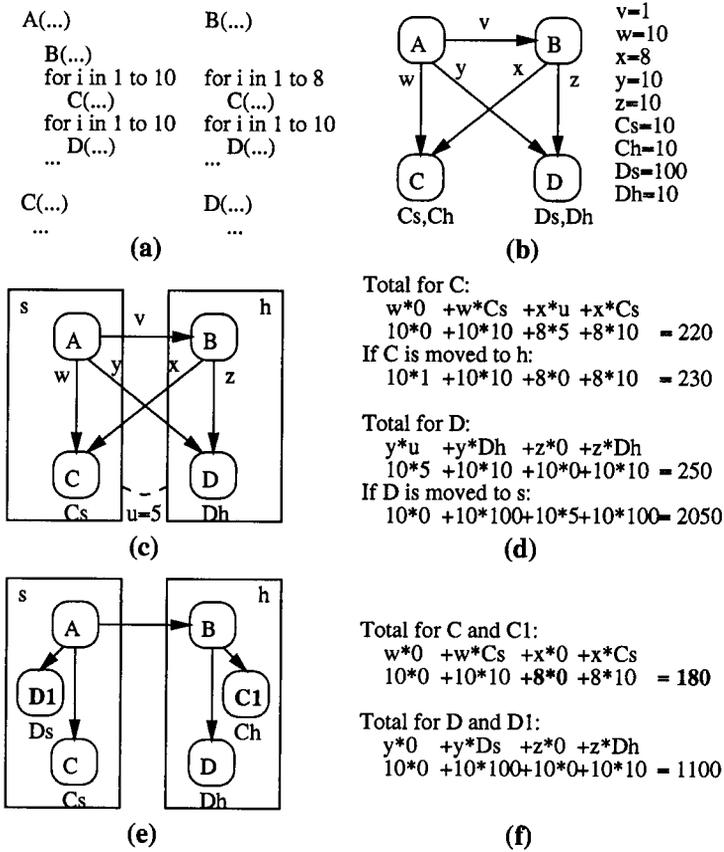
Fig. 1. Cloning example: (a) functional specification; (b) partially-annotated access graph; (c) first hardware/software partition; (d) time estimates for partition; (e) partition after cloning; (f) new time estimates after cloning.
