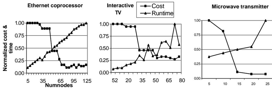
Fig. 8. Impact of different degree of clustering followed by  $N$ -way partitioning simulated annealing on three examples.
