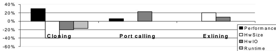
Fig. 7. Average improvements obtained by various procedure determination transformations followed by  $N$ -way partitioning (among hardware and software) using simulated annealing.
