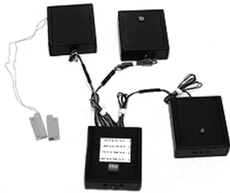
Figure 5: Garage Door Open At Night System built using eBlock prototypes.
