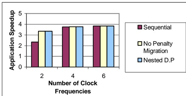
Figure 2. Results of the heuristics on a commercial quality video decoder. Compared to a single-frequency, single-coupling implementation of the accelerators, the heuristics improve the execution time by almost 4x.
