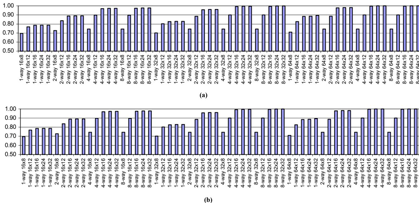
Figure 3: Sum of differences results for (a) Powerstone and (b) MediaBench. The x-axis shows the cache configuration with the number of ways followed by the cache size and frequency width in bits
