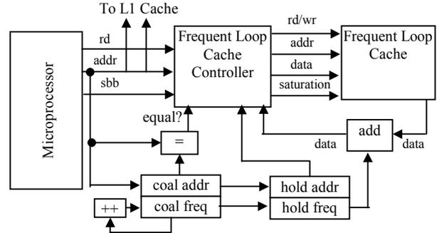
**Figure 5: Frequent loop detection architecture with backwards branch coalescing. Additionally, registers and arithmetic units have load and enable signals respectively.**
