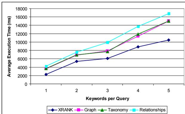
Fig. 4 Average Execution Time for Keyword Queries of different lengths.
