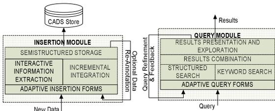
Figure 3: Architecture of Insertion and Query Modules.
