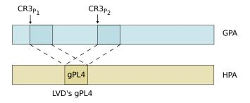
**Figure 3.** Cr3 remapping inside an LVD. The HPA page that contains the root of the LVD's page table (gPL4) is mapped at two GPA locations making it possible for two processes  $P_1$  and  $P_2$  to enter the LVD.
