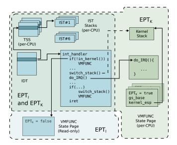
Figure 4. Data-structures involved in interrupt transition
