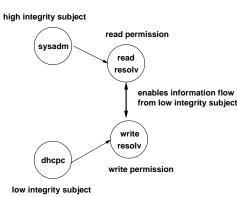
Figure 1: A direct conflict of a Biba integrity constraint caused by dhcpc writing to /etc/resolv.conf.
