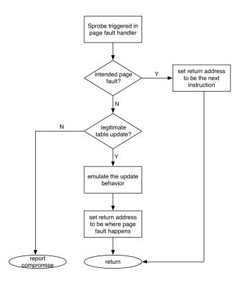
Fig. 4: SPROBE handling on data abort
