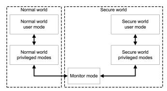
Fig. 1: TrustZone hardware architecture (from Figure 3.1 in [16])
