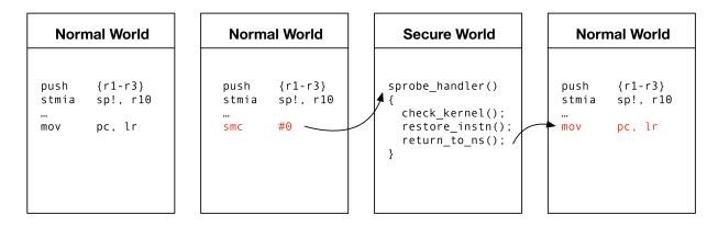
Fig. 3: World switches during SPROBE hit
