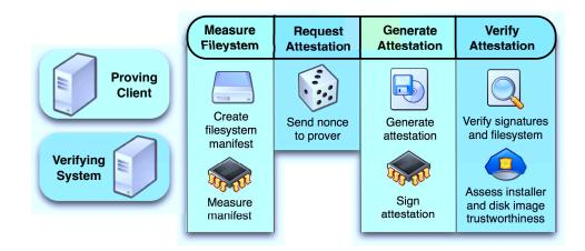
Figure 3: Timeline of the validation process. The filesystem on the proving client is measured to generate an attestation of the installed and current filesystems, which can be checked by the verifying system.
