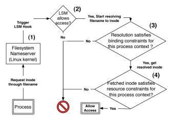
Fig. 2. Our prototype for the Linux filesystem enforces invariant *i-binding* at (3) and *i-resource* at (4).
