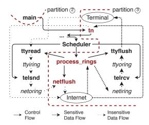
Figure 5: PDG and partitions for telnet.
