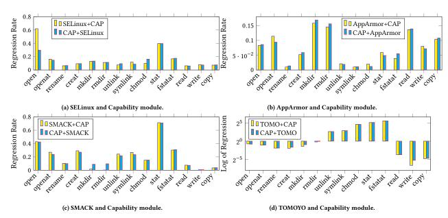
Figure 7: Overhead of Different Stacking Orders of LSM-based Security Modules. In regression rate, the lower the better. Tested with directory depth of one. (d) TOMOYO shows significant negative performance overhead especially, as there lacks cache for accesses, while SELinux, AppArmor and SMACK implement their own cache layers.
