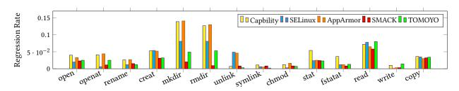
Figure 6: Performance Overhead of LSM-based Security Modules. Lower is better. Tested with directory depth of one.
