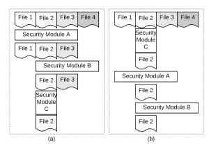
Figure 5: White-list Based Module Stacking. Stacking order matters to performance.
