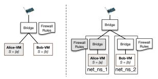
Figure 6: Isolating networking objects via network namespace.
