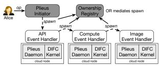
Figure 3: Overview: a user operation performed on Pileus.
