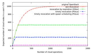
Figure 8: Expected number of cloud nodes in a user's TCB. The simulation consists of 1,000 cloud nodes. 5 are randomly picked each time to perform a cloud user's operation, and 10 operations are performed per second.
