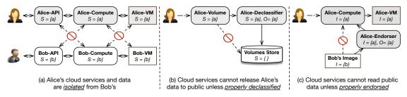
Figure 2: Decentralized information flow control examples in Pileus.
